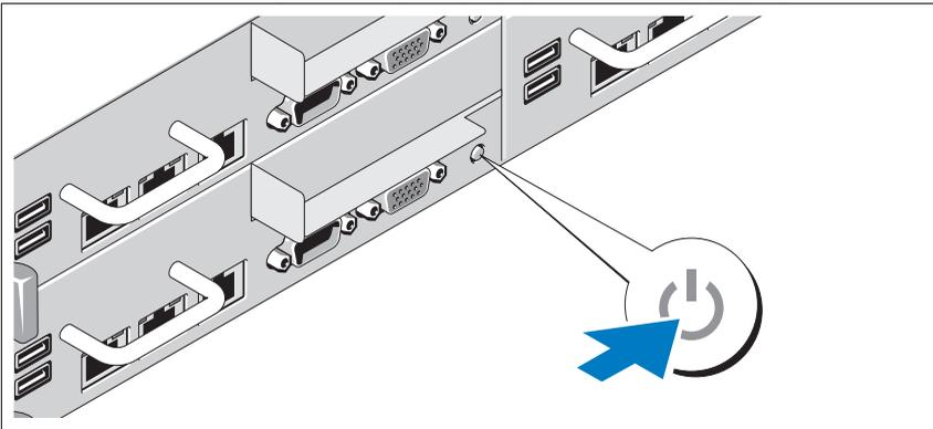
Press the power button(s) either on the front or back of the system and the monitor. The power indicators should light.
